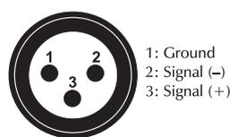
If you are using controllers with this occupation, you can connect the DMX output of the controller directly with the DMX input of the first device in the DMX chain. If you wish to connect DMX controllers with other XLR outputs, you need to use adapter cables.
