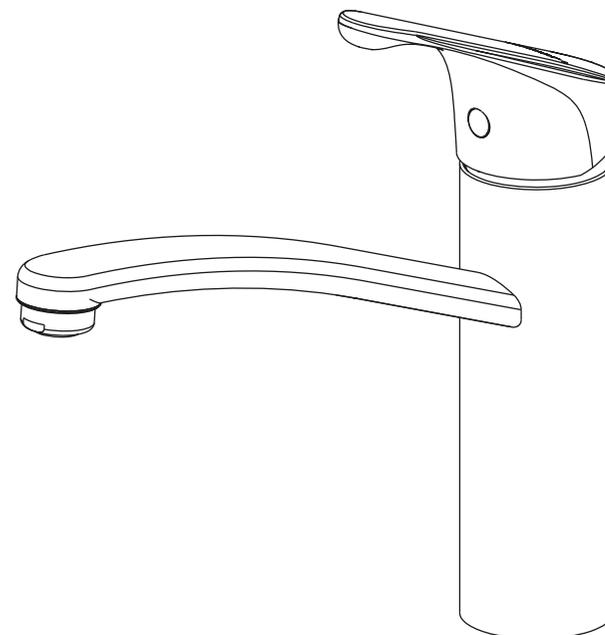
**CAUTION:** Always turn water OFF before removing existing or disassembling the faucet. Open faucet handles to relieve water pressure and insure that complete water shut-off has been accomplished.
