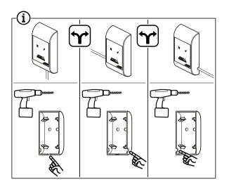
3. Make a hole in the frontplate. Run the cable through it.
