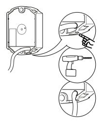
Make a hole in the bottom of the core unit and let the cable 2. run through it.
