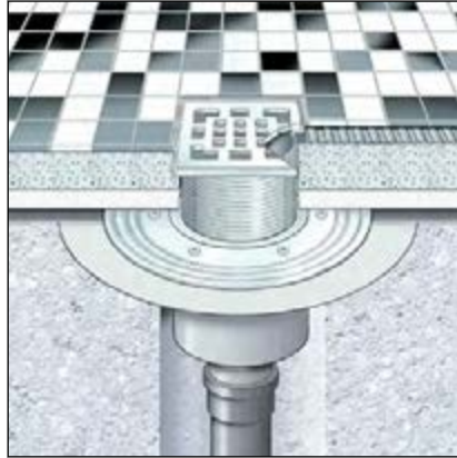
Fig. 3: Construction diagram of a conventional sealing
