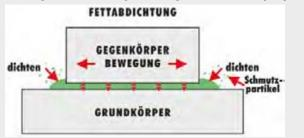
The grease forms a sealing "grease collar" between the basic body and counter body to protect against moisture and dirt particles. Dirt is prevented from entering the lubricating points, therefore ensuring longterm lubrication. The extended lubrication intervals are only possible with thorough pre-cleaning of the lubrication point. We therefore recommend cleaning thoroughly before each use with HHS® Clean.
