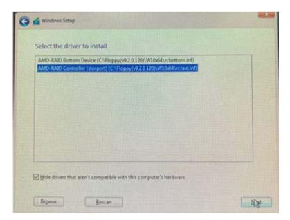
F. After RAID driver is loaded, the RAID disk will show up. Load the Third driver.
