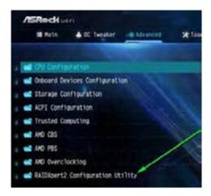
I. Go to Advanced → RAIDXpert2 Configuration Utility → Array Management, and then delete the existing disk arrays before creating a new array.
