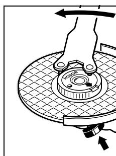
A properly attached, undamaged quick-clamping nut can be loosened by hand when turning the knurled ring in an anticlockwise direction. **Never loosen a tight quick-clamping nut with pliers. Always use the two-pin spanner.** Insert the two-pin spanner as shown in the illustration.
