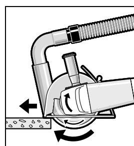
Switch on the machine and place the front part of the cutting guide on the workpiece. Slide the machine with moderate feed, adapted to the material to be worked.
