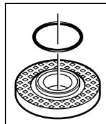
A plastic part (O-ring) is fitted around the centring collar of mounting flange **5**. **If the O-ring is missing or damaged,** the mounting flange **5** must be replaced before resuming operation.
