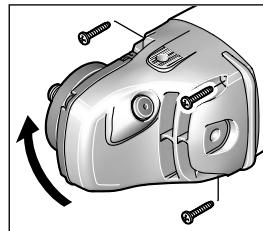
The machine head can be rotated with respect to the machine housing in 90° steps. In this manner, the On/Off switch can be brought into a more convenient position for special working situations, e.g., for cutting operations using the cutting guide with dust extraction protection guard **18** or for left-handed persons.
